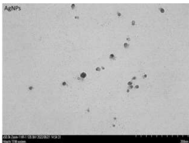
Figure 6: TEM image of AgNPs synthesized from 1.5 mM \text{AgNO}_3 and Cempedak bark extract (3:2 ratio), showing predominantly spherical nanoparticles with uniform distribution. Captured using Hitachi HT7700 at 120 kV and 50,000 \times magnification; scale bar = 200 nm.
