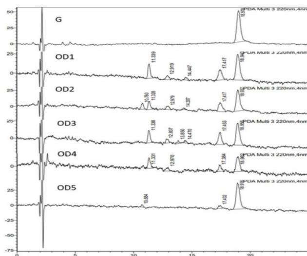
**Figure 4:** The HPLC chromatogram profile of the standard (-)- $\alpha$ -gurjunene(G) and test samples oleoresin (OD1-OD5) using an isocratic elution of 90%acetonitrile with a flow rate of 1.5 mL/min, injection volume 20  $\mu\text{L}$ , column temperature 25°C and UV detections at 220 nm. The retention time of (-)- $\alpha$ -gurjunene in all oleoresin samples were in the range of 18.916-18.982 min.
