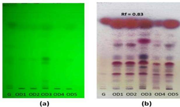
**Figure 3:** The normal phase TLC fingerprint of the *D. alatus* oleoresins detected under wavelength 254 nm (a) and spraying with anisaldehyde sulphuric acid reagent (b) using TLC normal phase TLC and mobile phase was hexane: ethyl acetate (8:2); Lane 1 is the standard (-)- $\alpha$ -gurjunene (G) and lane 2-5 were *D. alatus* oleoresins (OD1-OD5), respectively. The major compound in all sample is (-)- $\alpha$ -gurjunene with the  $R_f$  value at 0.83.
