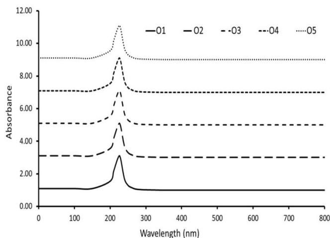
Figure 2: The UV-Vis spectra of the samples from *D. alatus* oleoresins (OD1-OD5) 100  $\mu$ g/mL (wavelength range 0-800 nm)
