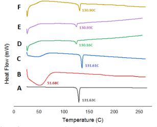
**Figure 2:** Thermogram of (A) piperine, (B) HPMC 2910, (C) physical mixture, (D) solid dispersion F1, (E) solid dispersion F2, (F) solid dispersion F3
