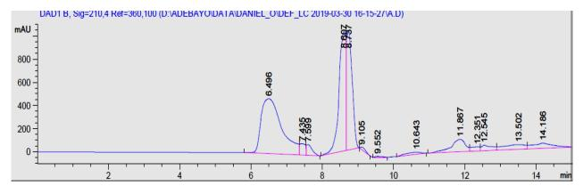
Figure 2: Chromatogram of Sample A recorded at 210nm and a flow rate of 0.25 mL/min. The chromatogram is offset for clarity.
