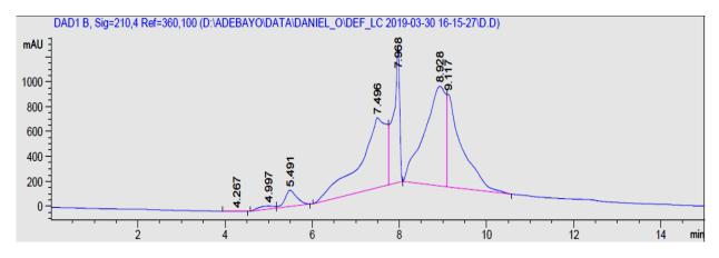
Figure 5: The chromatogram of Sample D was recorded at 210 nm and a flow rate of 0.25 mL/min. The chromatogram is offset for clarity. No peak for acrylamide was recorded.
