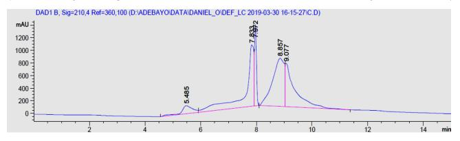
Figure 4: The chromatogram of Sample C was recorded at 210 nm and a flow rate of 0.25 mL/min. The chromatogram is offset for clarity. No peak for acrylamide was recorded.
