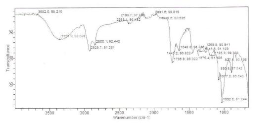
Figure 3: FTIR spectrum of isolated HPLC major peak
