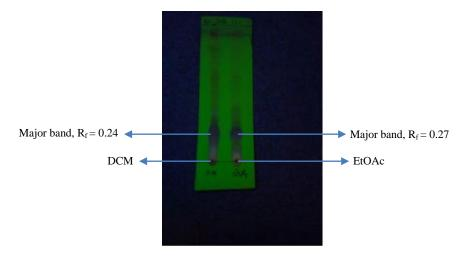
Figure 1: TLC profile of dichloromethane (DCM) and ethyl acetate (EtOAc) fractions viewed under a UV lamp at 365nm.
