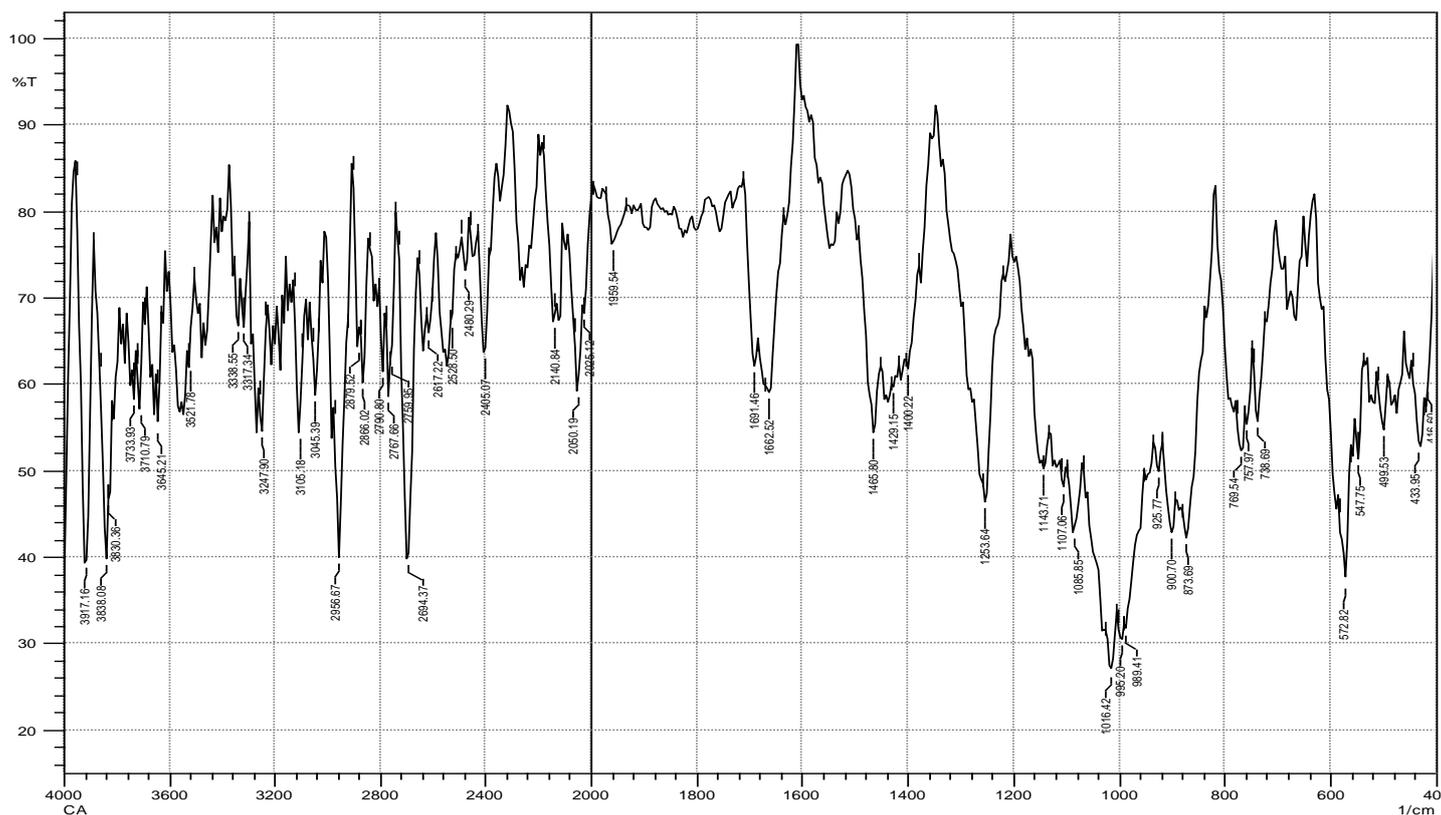
Figure 1: FTIR Spectrum of extracted *Anacardium occidentale* gum
