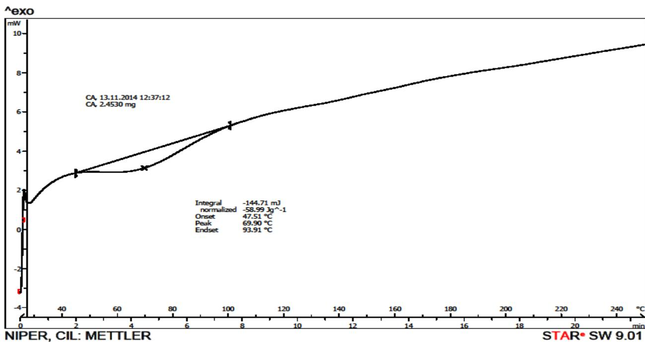
Figure 2: Differential Scanning Calorimetry (DSC) Thermogram of extracted *Anacardium occidentale* gum recorded in a dynamic nitrogen atmosphere (50 mL min<sup>-1</sup>), and at a heating rate of 2 °C min<sup>-1</sup>.
