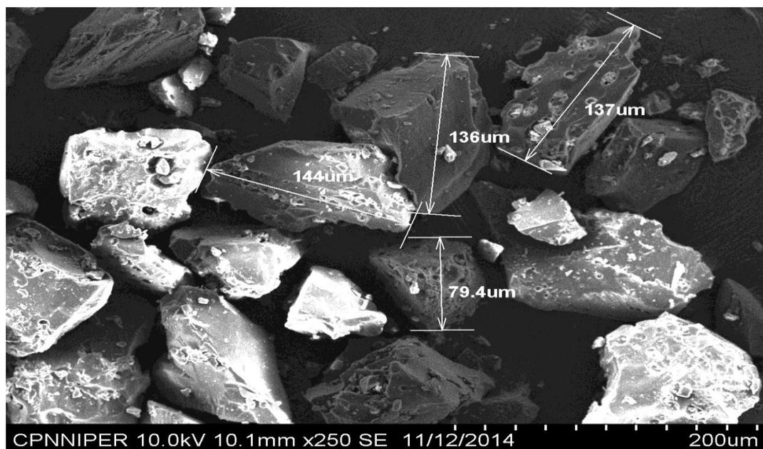
**Figure 4:** Scanning Electron Micrograph of extracted *Anacardium occidentale* gum @ x250 magnification
