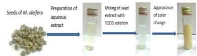
**Figure 1:** A scheme explaining the total procedure of nanoyttria synthesis using *Moringa oleifera* seeds
